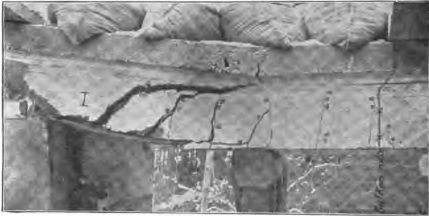
FIG. 119.—Failure cracks in the vicinity of the points of support of a concrete T-beam reinforced with only straight round rods.
