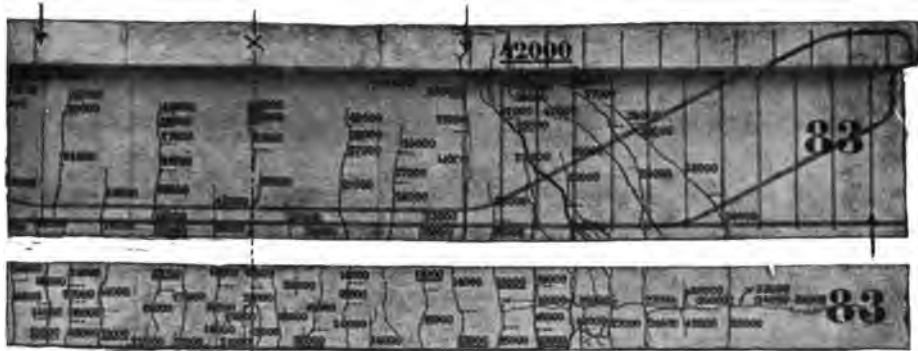
Fig. 166.—Side view, bottom, and cross-section of beams of T-section with one straight and four bent rods and with stirrups.
