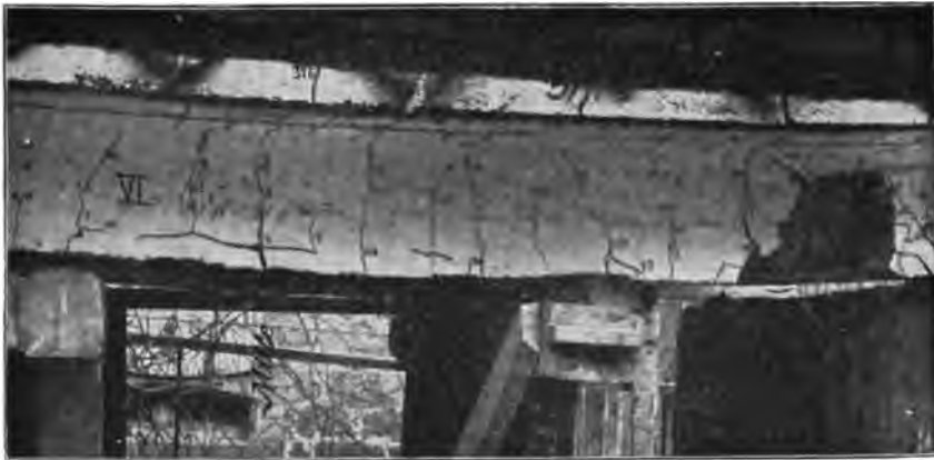
FIG. 150.—Beam VI, under the breaking load.
