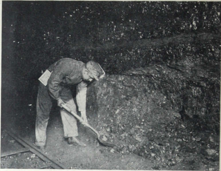
Lamp in use. The angle of illumination is well in excess of the 130 degrees required by the Government.
