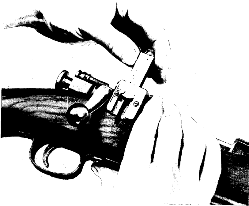
Figure 88 — Removing Rear Sight Elevating Slide From U.S. Rifle, Cal. .22, M2
