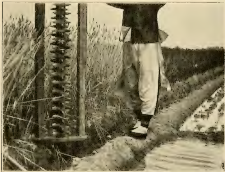
FIG. 144. — Form of revolving wooden harrow for fitting flooded rice fields preparatory to transplanting.
