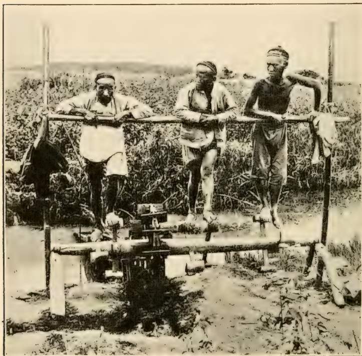
FIG. 36. - The wooden foot-power of China, used to propel the wooden-chain irrigation pump.
