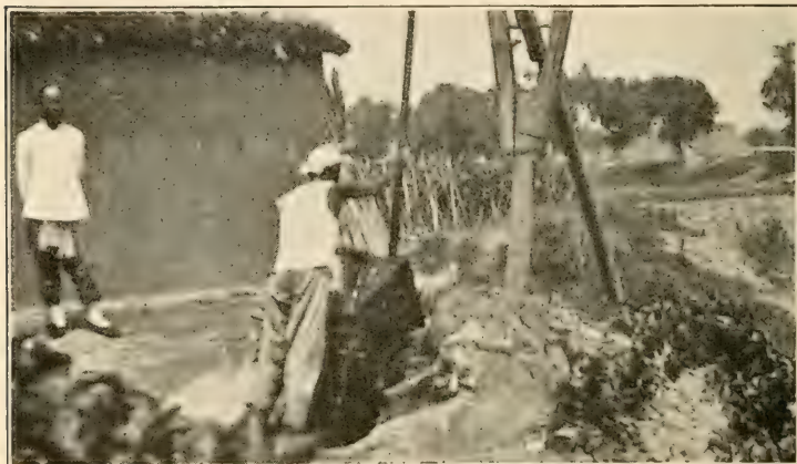
FIG. 152. — Well sweep and quadrangular conical water bucket used for irrigation in Chihli.
