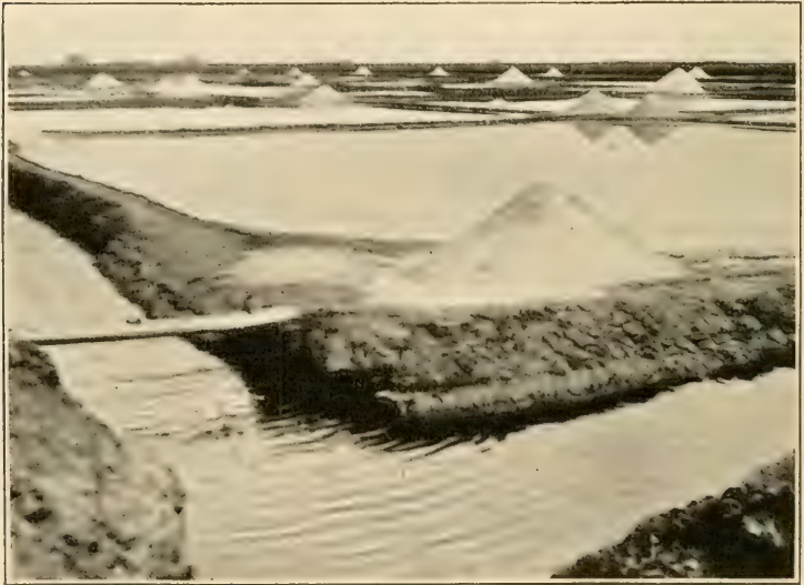
FIG. 176. — Near view of evaporating basins with piles of salt ready to be removed from the fields.
